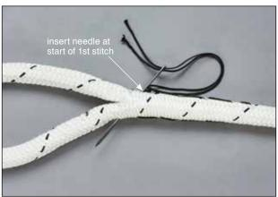
1.8 Insert both ends of the twine back in the needle. Insert the needle back into the body of the rope at the point where the first stitch starts. Angle the needle up towards the base of the eye so that the needle exits from the rope above the point where the first stitch is located on the opposite side of the rope.
