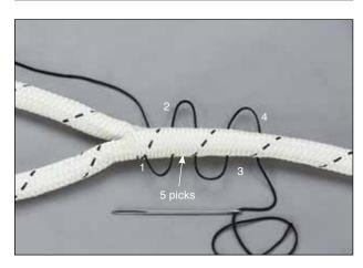
**1.2** Continue to stitch a total of 4 loops down the length of the splice following the same line of picks on each side of the rope. Each stitch should be 5 picks down from the point where the previous stitch comes out of the braid. This completes the first series of stitches. Do not pull the loops tight.
