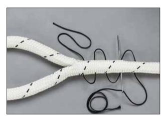
**1.3** For the second series of stitches, insert the needle back into the rope at the point where the last stitch on the same side is located and out on the opposite side of the rope where the previous stitch is located.
