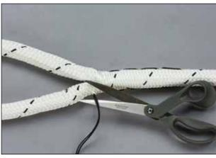
**1.10** Cut the excess ends of the twine close to the rope's surface.
