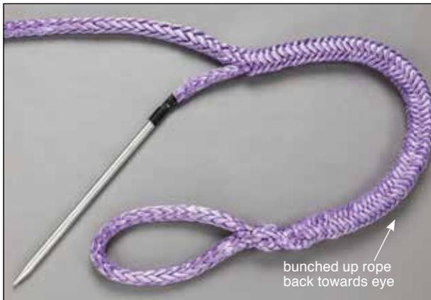
**3.8** Pull the remaining length of bitter end through the body of the rope. This will cause the rope to bunch up back towards the base of the eye and the brummel. Remove the fid from the bitter end.
