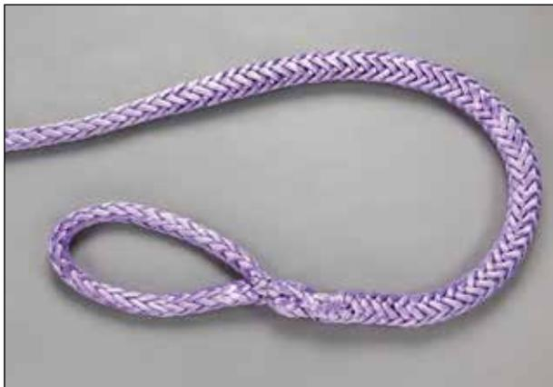
**4.5** The completed Buried Lockstitch Splice. Cross stitching is recommended, to prevent the splice from becoming loose or pulling out when the rope is not under load or when it might be mishandled. Please reference Cortland's Cross Stitching Instructions, document CT\_TL\_060\_0715.
