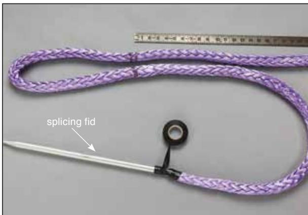
**3.2** Tape the splicing fid to the bitter end.
