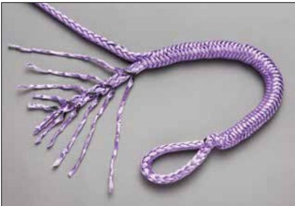
**4.2** Pull each of the marked strands out of the braid at the point where it has been marked.
