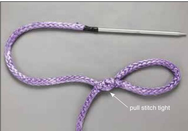
**3.6** Pull the fid and bitter end all the way through so that the resulting loop or “stitch” is pulled tight.
