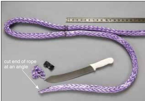
**3.1** Remove any tape from the bitter end of the rope and then cut the end of the rope at an angle.
