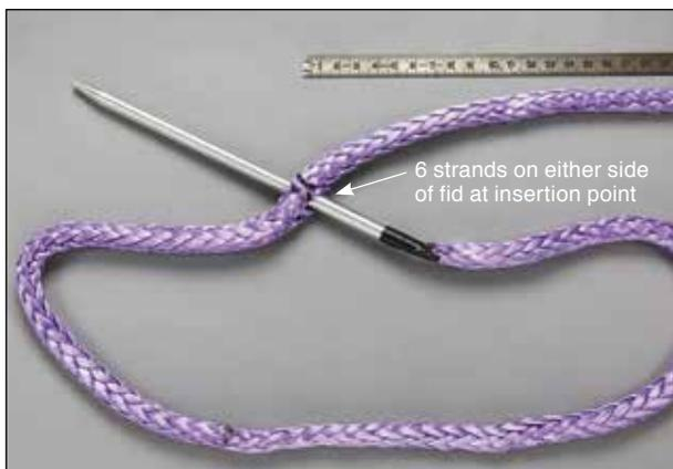
**3.3** Insert the fid directly through the body of the rope at Mark 2. The fid should be inserted between strands.
