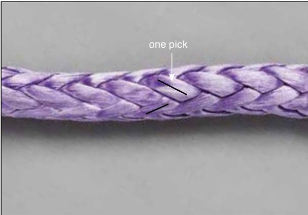
**NOTE:** A pick is a point on the braid in which one strand in the left or “s” direction crosses over or under a strand in the right or “z” direction. This is illustrated in the image to the left.
