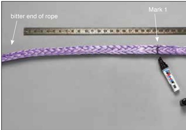
**1.1** Lay the end of the rope out straight on the work surface. Starting at the bitter end of the rope, measure a distance down from the end equal to two fid lengths for Type 1 ropes and three fid lengths for Type 2 ropes. The fid length for the specific rope size can be found in the table on the preceding page.
