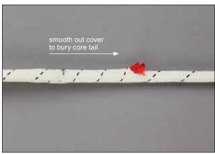
**4.5** Once the core strands are tapered, smooth out the bunched up section of cover from the base of the eye towards the tapered ends of the core to bury the exposed ends of the core back inside the body of the rope.
