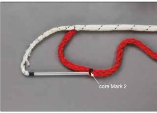
**3.5** Insert the fid into the core at Core Mark 2 (step 2.4) in the direction of the anchor point.
