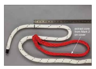
**2.3** Extract the core braid at Mark 2 on the cover, pulling the core out of the cover from Mark 2 towards the hitch knot at the anchor point. Pull the bitter end of the core out of the cover braid as well.
