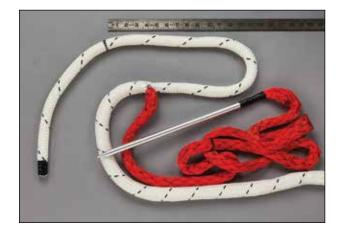
**NOTE:** A pick is a point on the braid in which one strand in the left or "s" direction crosses over or under a strand in the right or "z" direction. This is illustrated in the image to the left.
