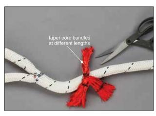
**4.4** Pull the core tail out from the cover about 1/3rd of a fid length and cut off the excess core tail at the mark that was just made. Then taper the exposed end of the core.
