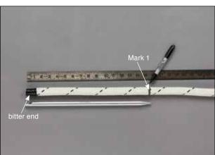
**1.1** Secure the rope to a sturdy post or anchor point by tying a hitch type knot 7–10 fid lengths down from the free end of the rope (the bitter end). If possible, insert a large sewing needle or pin through the rope just in front of the knot to assist in holding the cover and core together.
