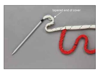
**3.4** Remove the fid from the bitter end of the core and tape it to the tapered bitter end of the cover.
