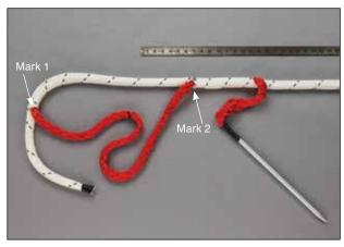
2.7 Milk the fid through the cover braid until it reaches the point where the core was extracted from the rope (Mark 2 on the cover). With the tip of the fid positioned at the point of extraction, carefully continue to push the fid past Mark 2. Avoid snagging the core inside the cover with the tip of the fid. Continue to push the fid about 1/3 fid length past Mark 2 and then exit the fid and core through the cover.
