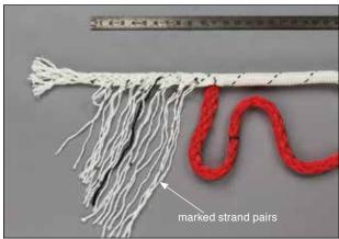
**3.2** Pull each of the marked strand pairs out from the end of the cover braid.
