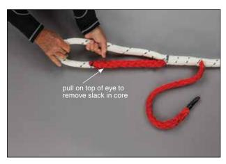
**4.1** Pull on the cover side of the eye to remove any slack or bunching of the exposed section of core.
