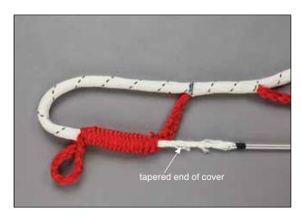
**3.7** Pull the fid out of the core exposing the entire fid and as much of the cover tail as possible. This will require bunching up the core back toward Core Mark 2.
