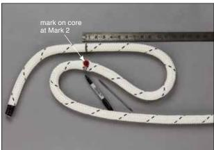
**2.2** Use a large needle, fid or similar tool to separate the cover yarns at Mark 2, exposing the core. Make a mark on the exposed core with the marker pen. This is Core Mark 1.
