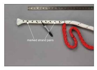
**3.1** Remove any tape around the bitter end of the cover. Working from Mark 1 on the cover count 5 picks (strand pairs) toward the bitter end of the rope and mark the 5th pair to form a V shaped mark on the cover. Then count down 4 picks and mark the 4th pair. Alternate counting and marking the 5th and then 4th pick (strand pair) until you reach the end of the rope.
