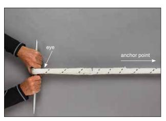
**4.6** To finish the splice, hold the top of the eye and pull against the anchor point. This will assist in removing any remaining slack in the rope and burying the exposed core in the eye. Cover slack can also be removed by milking the cover back towards the eye from the anchor point while keeping the rope under some slight tension.
