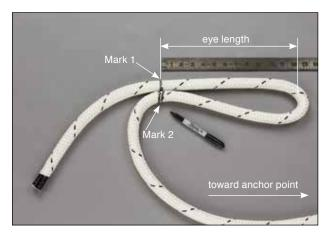
**Quality Check** Ensure accurate markings in Step 2. Inaccurate marks will directly affect the quality of the splice.
