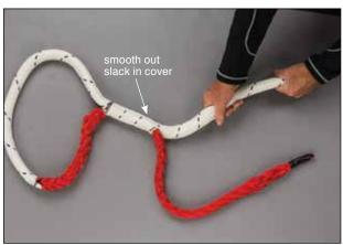
4.2 Working from the standing part of the rope attached to the anchor point, milk or smooth out any slack in the cover towards the base of the eye. Continue to alternate between Step 4.1 and 4.2 until all slack is removed from the cover and the exposed core has been completely buried in the cover in the eye.
