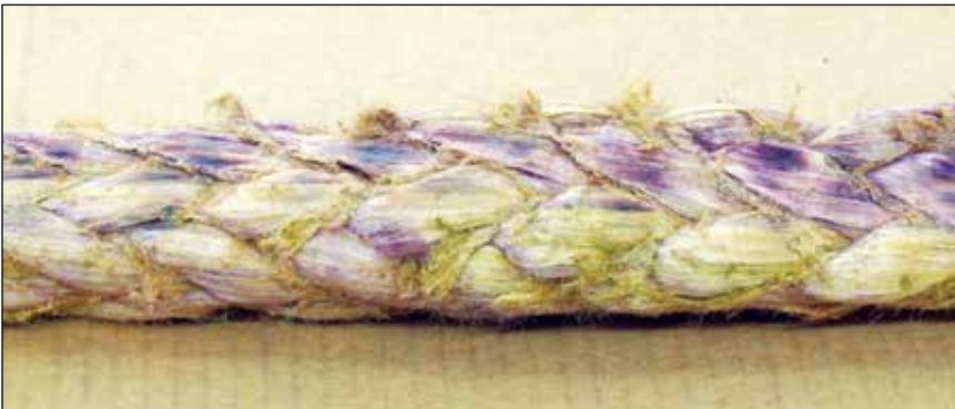
Example of burned and partially melted fiber
