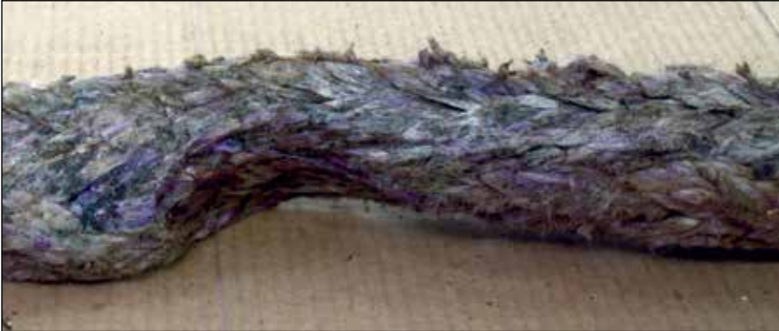
Example of burned and excessively melted fiber
