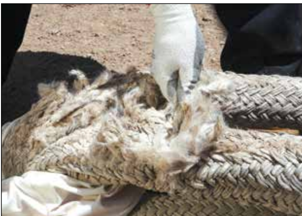
Excessive cutting or wear on braided UHMWPE wear protection. If synthetic rope is visible through cut protective sleeve, inspect rope component also.
