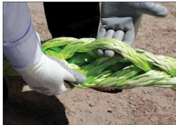
New braided synthetic rope component. No external rope strand or rope core wear or damage.
