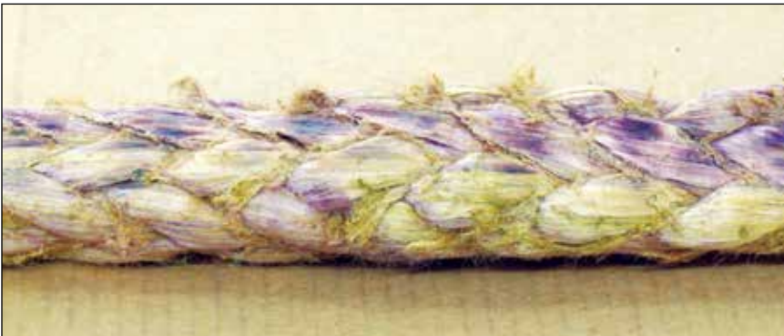
Example of burned and partially melted fiber
