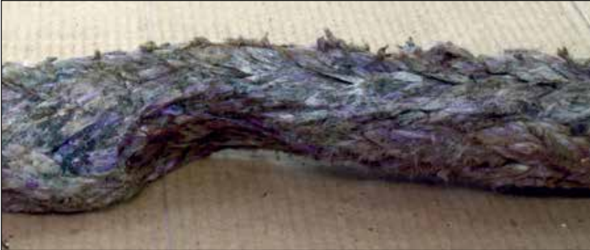
Example of burned and excessively melted fiber
