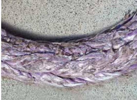
Inspect for excess surface wear on rope
