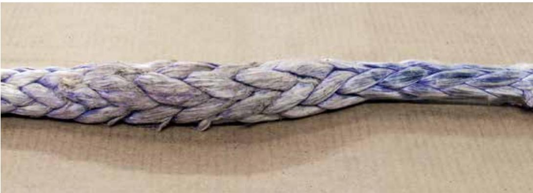
Plasma® 12x12 rope slings are manufactured with balanced yarn and strand construction. Distorted and/or damaged yarns and strands usually occur in most applications. Ropes exhibiting areas of severely distorted construction or yarn damage should be repaired or retired from service.
