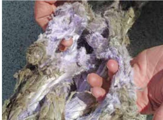
Excessive **interior** abrasion wear
