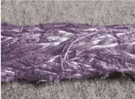
Excessive **exterior** abrasion wear
