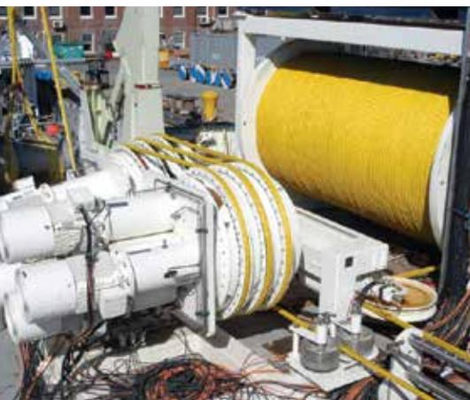
**Super Wide Tow Rope** Probably the most critical rope within the seismic array, super wide tow ropes need to cope with high levels of tension-tension and cyclic bend fatigue.
