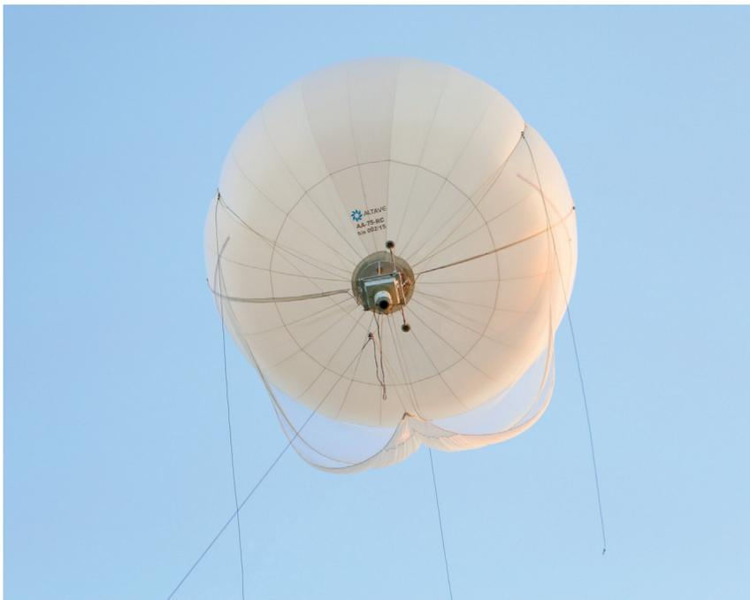
Altave's surveillance balloon with Cortland's aerostat tether attached
