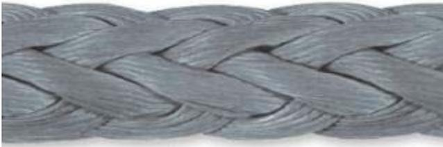
Figure 1. Example of typical 12 x 1 design HMPE rope; each strand with “singles” twisted yarns
