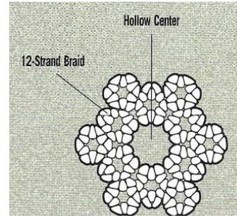
Figure 3. Cross section view of 12 x 12 design rope
