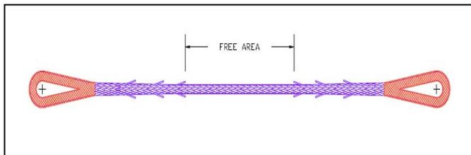
Figure 8. Drawing of Plasma® 12 x 12 eye-and-eye sling with Moran 5/4/3 splice and “free area” between bases of the splices
