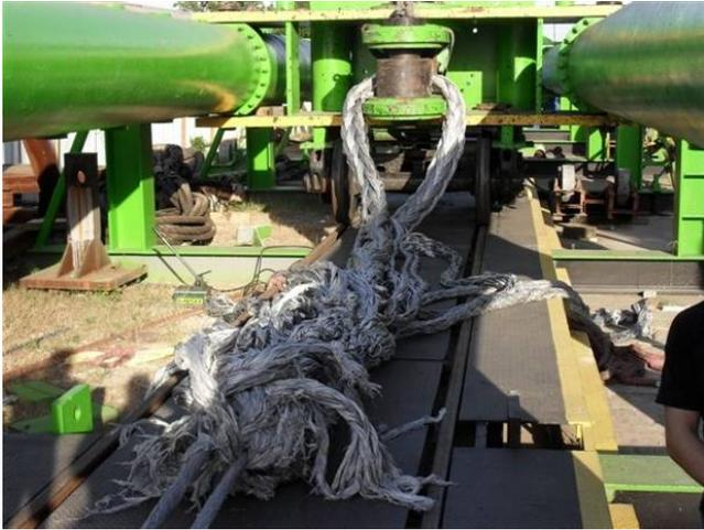
Figure 10. 168mm diameter Plasma® 12 x 12 rope sample after destructive test. Note at bottom left of photo that two of original 12 strands are still intact.
