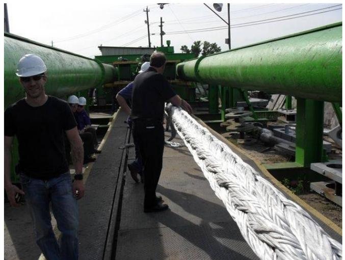
Figure 9. 168mm diameter Plasma® 12 x 12 tensioned on test bed
