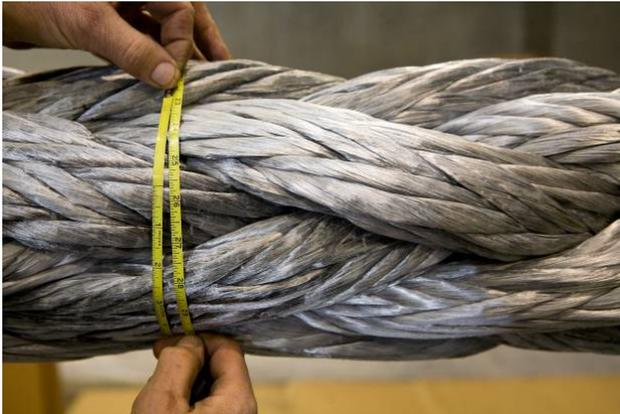
Figure 7. O.D. measurement of 168mm diameter Plasma® 12 x 12
