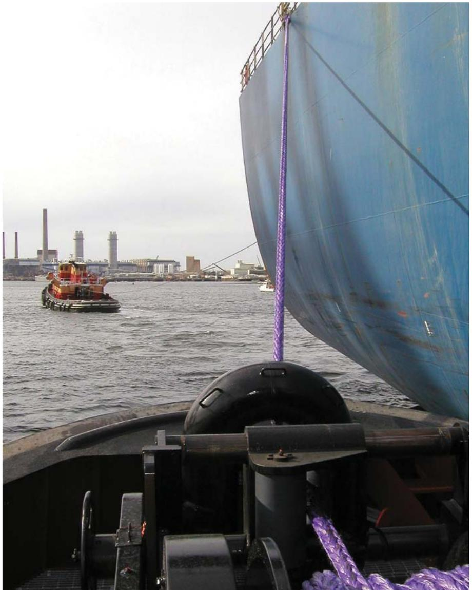
▲ Cortland's Plasma line being used on a tug alongside a vessel
