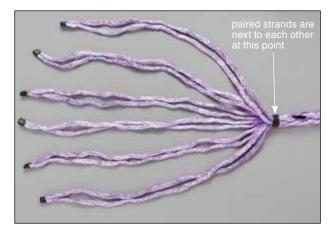
**2.1** The rope is made up of six "S" or left direction strands and six "Z" or right direction strands. One "S" and one "Z" strand should be combined together to form a strand pair. The paired "S" and "Z" strands should be adjacent to each other at the point where they exit from the tape placed around the circumference of the rope. After an adjacent "S" and "Z" strand have been paired up, tape the two strands together. A total of six strand pairs will be formed in this manner.
