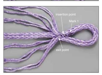
**3.1** While keeping the shape of the soft eye, form an opening between two adjacent strands at the Insertion Point to allow a Strand Pair to be inserted. A Swedish Fid or similar tool may be used during this process. If a Swedish Fid is used, insert it at the Exit Point under one of the Strand Marks and bring the tip of the fid out at the Insertion Point between the two adjacent strands.
