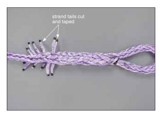
**4.4** After all of the tucks have been completed the ends of the strands can be cut off at a point about one rope circumference in length away from the point where they exit from the last tuck. The ends of the strands should be tightly taped after cutting.
