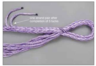
**4.2** A total of five complete tucks will be made with each tucking strand. When the five tucks are completed six of the individual tucking strands will be located slightly further down the body of the rope than the other six strands.
