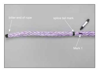
1.1 Mark a length 18 picks down from the bitter end of the rope and put a piece of tape tightly around the circumference of the rope at this point. This is the Splice Tail Mark. A pick is a point on the braid in which one strand in the left or "S" direction crosses over or under a strand in the right or "Z" direction, as shown in the photo. Next, count down one additional pick and mark with a black marker. This is Mark 1.
