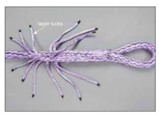
**4.3** The final set of two taper tucks is performed in the same manner as the previous tucks by using every other individual tucking strand. As before, select any one individual strand and perform two tucks (over one strand and under one strand) down the length of the rope. Then skip every other stand and do two tucks with the remaining five strands.
