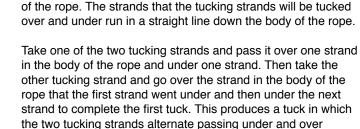
**4.1** Select any one Strand Pair and remove the tape holding the two strands together to form two individual tucking strands. The tucks will be made with each individual strand down the length
