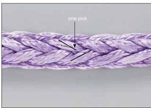
**1.2** Unlay the end of the rope and tape the end of each strand. Continue unlaying the rope back to the piece of tape at the Splice Tail Mark.
