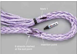
**2.2** Using Mark 1 as a reference point, form the size of eye required. When forming the eye make sure that there is no twist in the rope. When the eye is formed to the desired size make a mark on the body of the rope opposite to the Mark 1. This is the Insertion Point.
