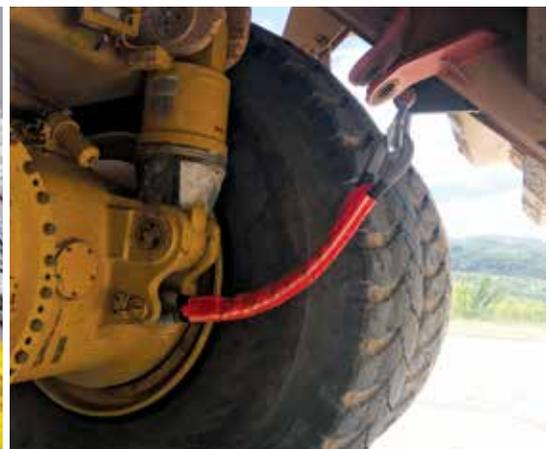
Designed to replace steel, synthetic rope solutions are now globally accepted as recovery and tow cables, lifting slings, and winch lines
