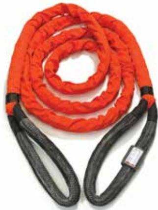
Cortland's recovery and tow cables are typically supplied in an endless loop (grommet) fabrication with eye terminations each end. The rope is not affected by water, is very cut resistant and has excellent UV resistance; it also offers effective strength retention in the hottest or coldest environments.
