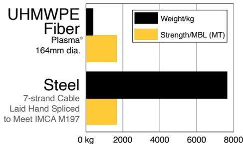
Not all modern high performance synthetic solutions are designed and produced the same. While raw material choice, quality, construction, twist, braid levels, and coatings vary by manufacturer, we are proudly innovative in our fiber solution design and performance. Cortland fabricated ropes will produce weight, strength and product performance which cannot easily be compared with other manufacturers.
