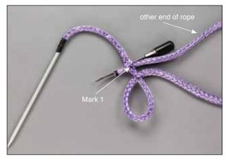
**3.5** Use a 2nd fid to create an opening directly through the bitter end at Mark 1.
