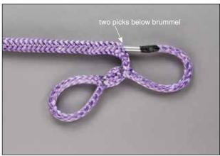
**3.7** Insert the fid and the bitter end back into the body of the rope at a point two picks below the bottom of the last brummel.
