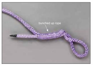
**3.9** Pull the remaining length of bitter end through the body of the rope. This will cause the rope to bunch up back towards the base of the eye and the brummel. Remove the fid from the bitter end.
