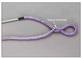
**3.6** Insert the opposite end of the rope through the opening and pull the entire length of rope through until the resulting loop (brummel) below the base of the eye is tight.
