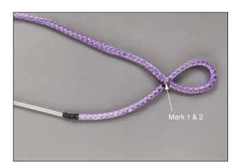
**3.4** Pull the fid and bitter end through until Mark 1 is visible just past the exit point at Mark 2.
