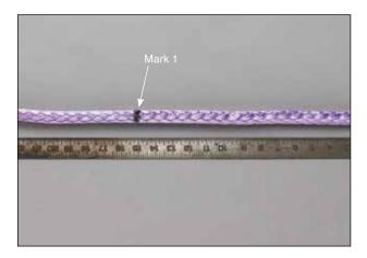
1.1 Lay the end of the rope out straight on the work surface. Starting at the bitter end of the rope, measure a distance down from the end equal to one fid length for Type 1 ropes and two fid lengths for Type 2 ropes. The fid length for the specific rope size can be found in the table on the preceding page.
