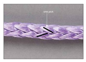
**NOTE:** A pick is a point on the braid in which one strand in the left or "S" direction crosses over or under a strand in the right or "Z" direction, as shown in the image to the left.
