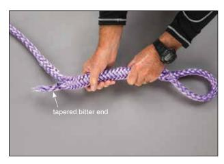
**4.4** Working from the base of the eye smooth out the bunched up rope away from the eye to bury the tapered bitter end back inside the body of the rope.
