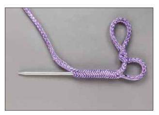
**3.8** Push the fid down the center of the rope for a distance of 1-1/2 fids for Type 1 rope and 2-1/2 fids for Type 2 rope. Bring the tip of the fid out of the body of the rope at this point.
