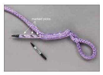
**4.1** Working from the bitter end, count 3 picks (strand pairs) away from the end and mark the 3rd pair to form a V shaped mark on the rope. Then count 2 more picks up the rope and mark the 2nd pair. Alternate counting and marking the 3rd and then 2nd picks for a length of about 1/3 fid away from the bitter end.
