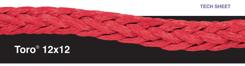
Toro® 12x12 is a 12-strand braided rope in which each of the 12 strands is, in turn, a 12-strand rope, or braided primary strand. Toro is manufactured from high tenacity High Modulus Polyethylene (HMPE).
