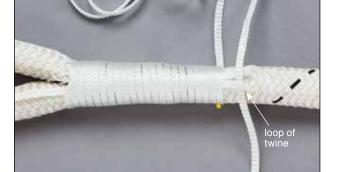
5.5 Insert the end of the twine through the exposed loop.
