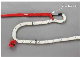
3.2 Insert the fid at Mark 1 on the core and push the fid through toward the bitter end, exiting the core at a point approximately 2/3 of a fid length down from the insertion point. Pull the fid out of the core exposing the entire fid and as much of the cover tail as possible. This will require bunching up the core back toward Extraction Point 1.
