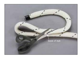
**5.1** Cut rope cover tail diagonally starting at the core entry point at the base of the eye. The length of the cover tail after cutting should be at least 3" (76mm) at its longest point.
