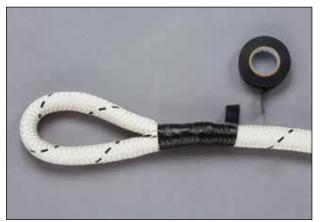
**5.2** Tape over the cover braid tail from the base of the eye to the end of the cover tail.
