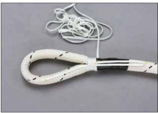
5.4 Starting at the base of the eye begin to wrap the standing part of the twine tightly over the taped and spliced area of the rope. Avoid gaps between adjacent wraps of the twine. Continue to wrap the twine down to a point just before the loop of twine at the end of the splice.
