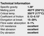
\* value based on data supplied by the fibre manufacturer for new, dry fibre
